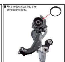
Fix MD2 C48 rear derailleur cage into derailleur's body. Please lock the spring on the inner latch position of derailleur's body.
