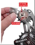
■ Put the extension spring on the adapter of MD2C48.
